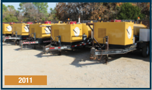
(6) VAC-TRON HYDRO EXCAVATORS
